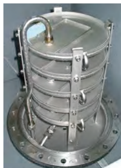
Figure 9. EMPA liquid sorption reactor first stage (left, upper dishes covered with insulation) and one of the heat/mass exchangers of the second stage (right).
