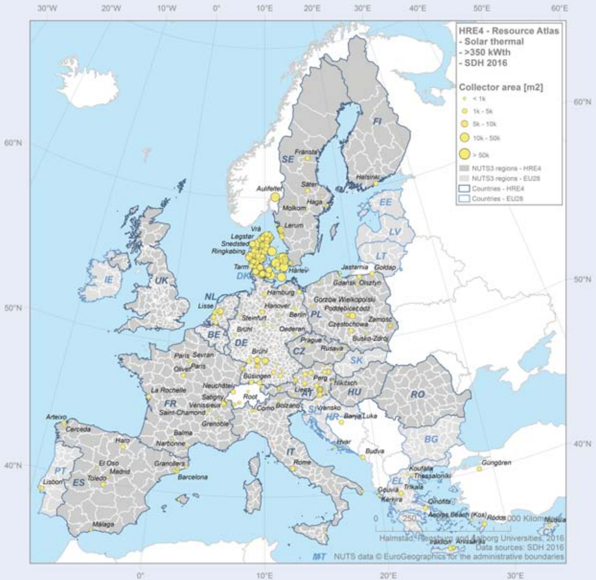
Figure 7: Solar district heating systems > 500 m 2 (> 350 kW th ) in Europe. (Source: EU-project Heat Roadmap Europe)
