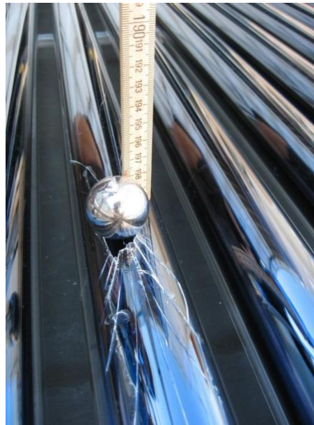
Figure 3: Damaged collector after steel ball impact test
