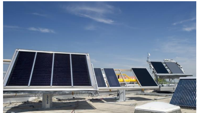
Figure 1: Outdoor exposure at the testing facility of Fraunhofer ISE
