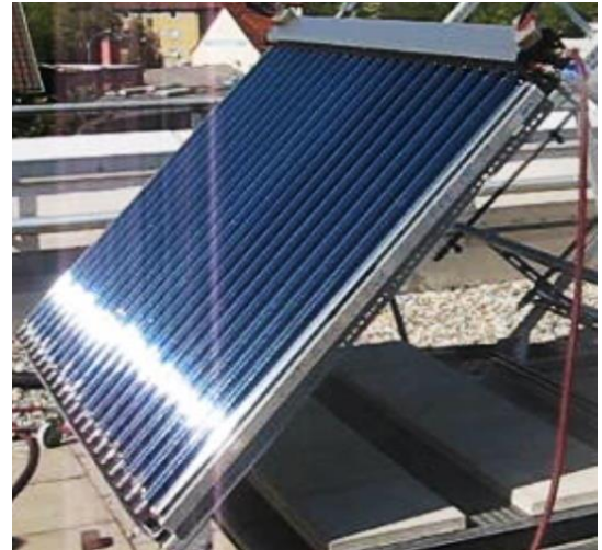
Figure 1: Internal thermal shock test; Fraunhofer ISE
